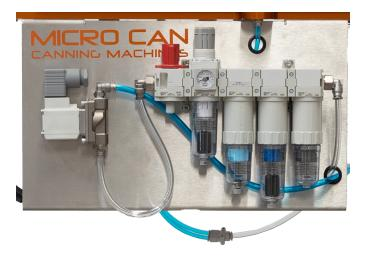
A water option is available as the standard unit comes fitted with a drip tray. The customer is responsible for the quality of the water that is connected to the Rinser. The connection is via a 10mm push fit fitting to a stainless-steel solenoid valve.
